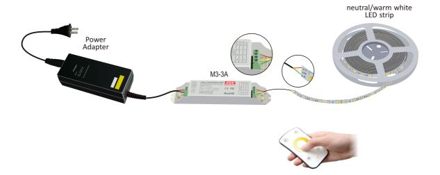
Note: Connection according to the strip with the actual definition of location wiring, line color only for reference.
